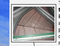
The volatile organic compounds VOC contained in the laden air flow are concentrated by adsorption in a zeolite-based rotor-concentrator. The cleaned air flow is delivered directly to the exhaust stack. The pollutants concentrated in the rotor-concentrator are desorbed and finally treated by a thermal oxidizer with reduced size.
