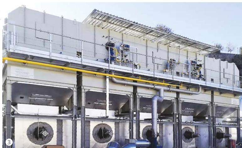
Figure 3: A regenerative thermal oxidiser (RTO).
